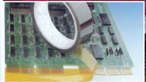
Finger masking with polyimide tape
